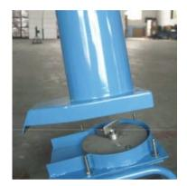
3) Remove the rotating plate fixing the cutter plate. Then take the cutter plate (10) from the base plate (15) and clean it.
